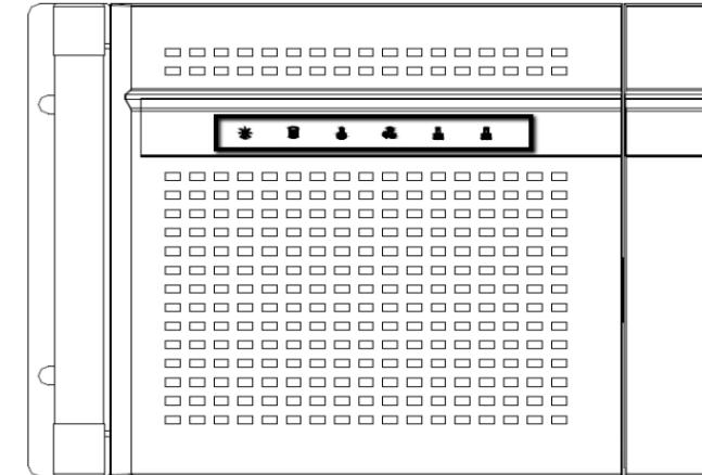
**Momentary Power switch:** Press this switch to turn the system power on or off. Please use system shutdown or press this switch for few seconds to turn off the system ATX power.
